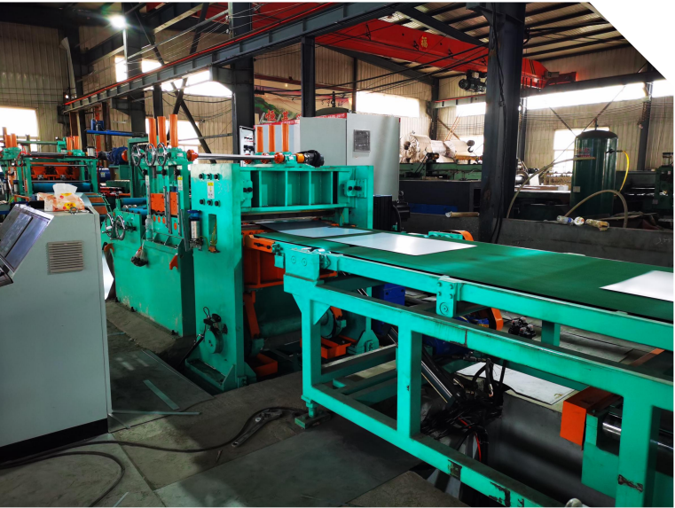
Cut to length Line
