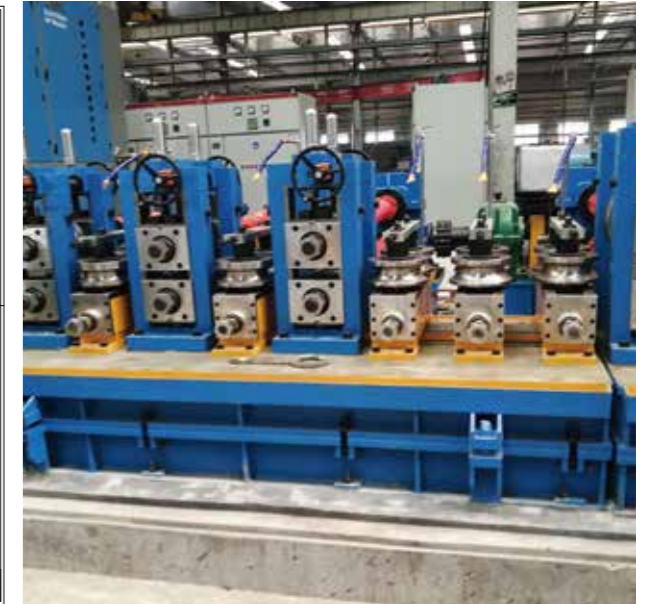
▶ Round Pipe: \phi 32-89(\text{mm}) Square/Rectangular: 25*25-70*70(\text{mm}) Pipe Thickness: 1.0-4.5(\text{mm}) Production Speed: 60-100(\text{m}/\text{min})
