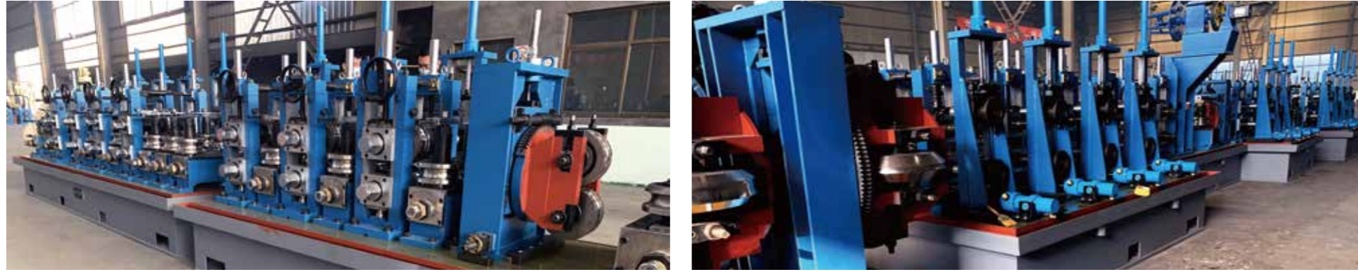
▶ Round Pipe: \phi 32-127(\text{mm}) Square/Rectanglar: 50*25-140*60(\text{mm}) Pipe Thickness: 0.9-4(\text{mm}) Production Speed: 20-80(\text{m}/\text{min})
