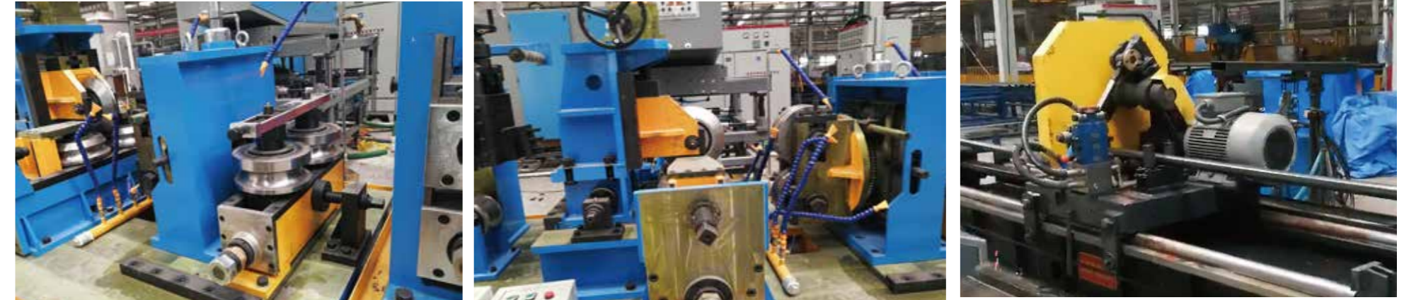
▶ Round Pipe: \phi 32-89(\text{mm}) Square/Rectangular: 25*25-70*70(\text{mm}) Pipe Thickness: 1.0-4.5(\text{mm}) Production Speed: 60-100(\text{m}/\text{min})
