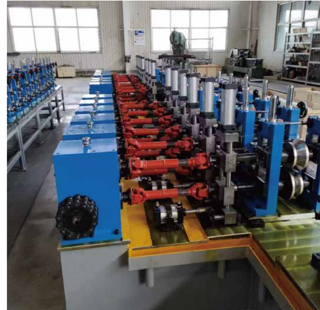
▶ 传动轴快换 & 工作台快换 Drive shaft quick change & table quick change
