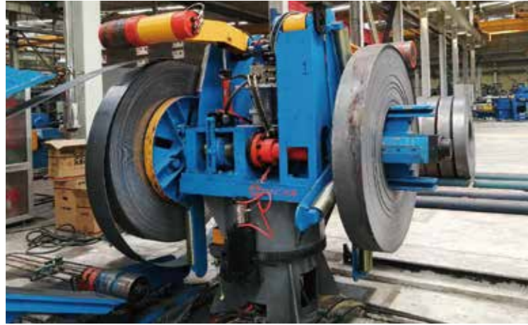
▶ 双锥液压 Double cone hydraulic T ≤ 4t
