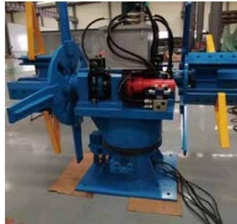
▶ 双锥液压 Double cone hydraulic T ≤ 4t
