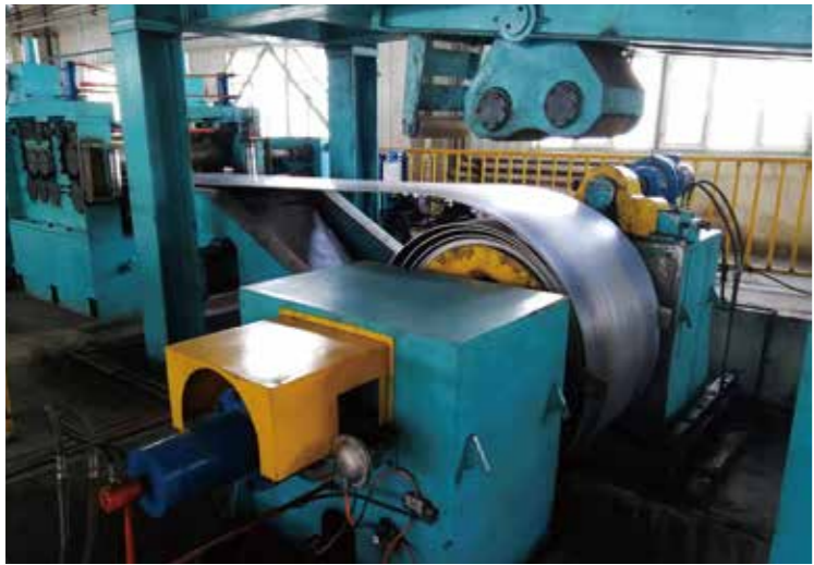
▶ 对锥液压 Double cone hydraulic T ≤ 25t
